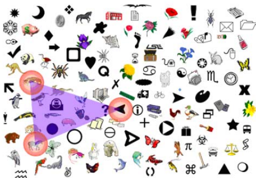
Figure 2. A shoulder-surfing resistant graphical password scheme [12]
