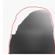
Fig. 13. Smearing at the tip of the finger. The red line indicates the estimated border outline of the finger, not visible due to a saturation trail.
